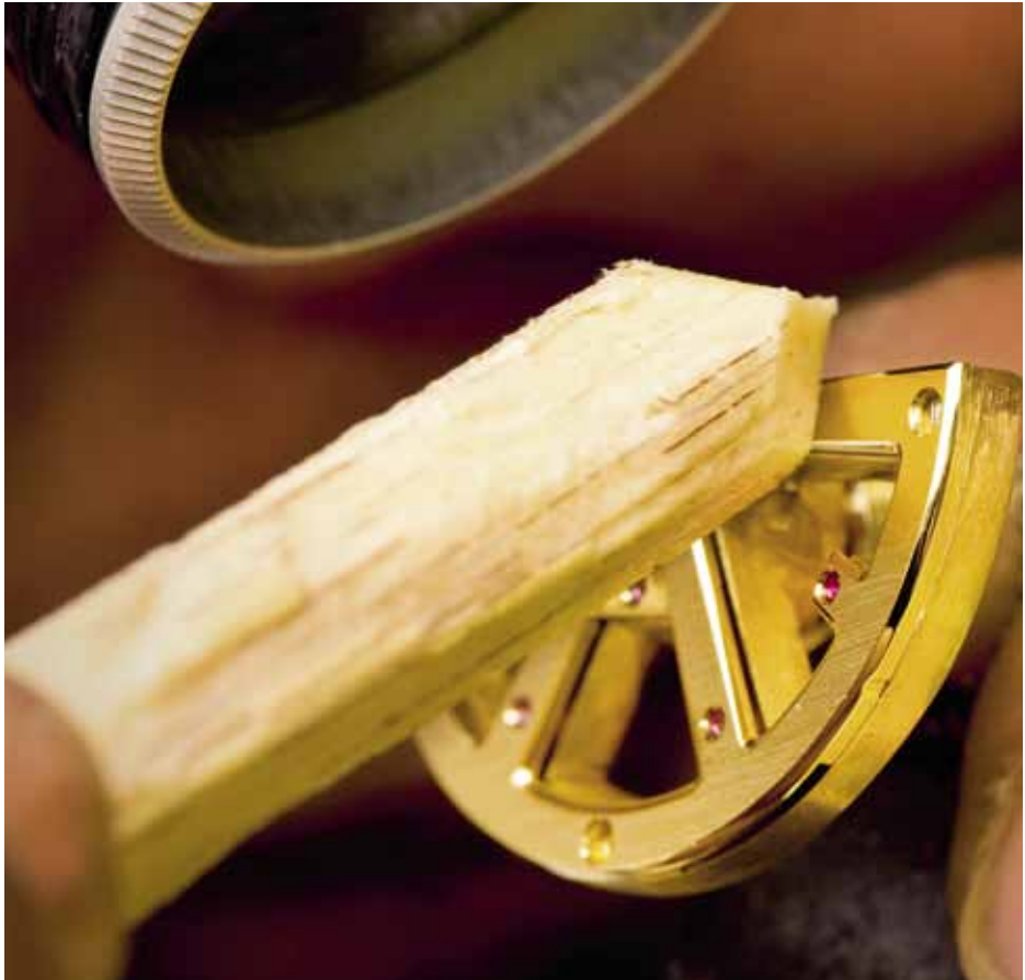
Final step of polishing the bridges
