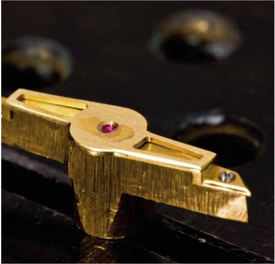
Bevelling of the seconds bridge
